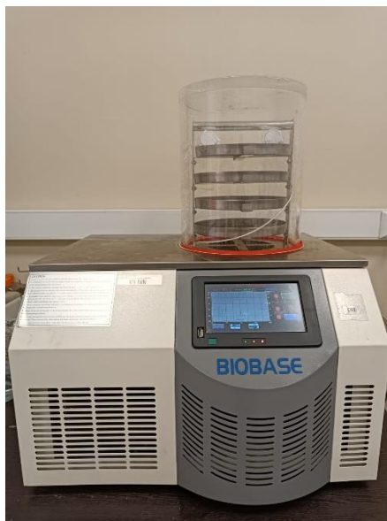
Figure 2.3: The lyophilizer device used for freeze-drying method
