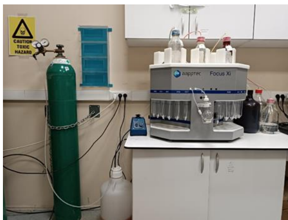
Figure 2.1: Automated peptide synthesis device used for performing solid phase peptide synthesis
